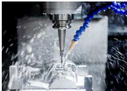
Fig 1: Highly accurate tooling is required to produce wax patterns
