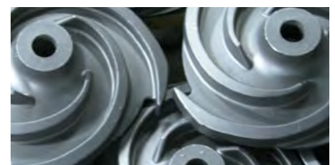
Fig 7: Silica Sol castings deliver tight tolerances and excellent as-cast surface finishes
