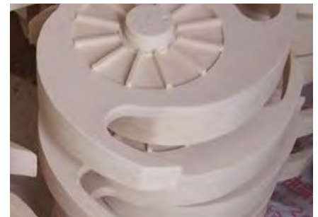
Fig 2: Wax patterns are carefully checked for imperfections
