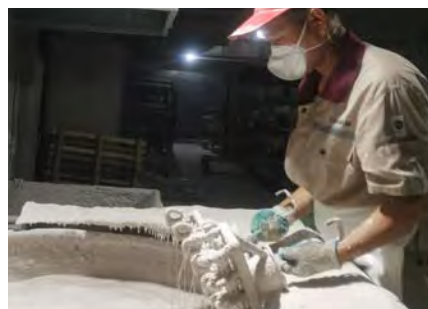
Fig 3: Wax pattern ‘trees’ are created and dipped in ceramic slurry
