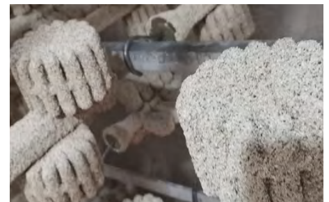
Fig 6: Silica Sol can handle the very high temperatures required for Stainless Steel castings
