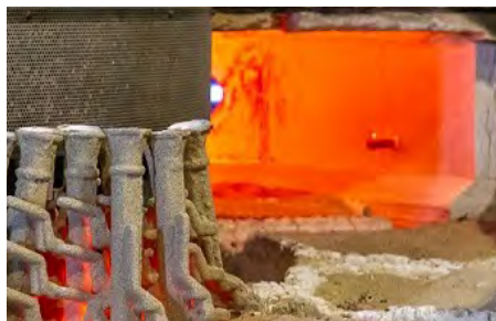
Fig 5: Silica Sol moulds are baked to eliminate moisture and remove any residual wax
