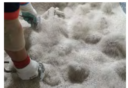
Fig 4: Slurry-coated wax trees are dipped in silica sol zircon sand
