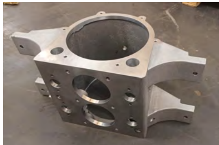
The new crankcase was cast in aluminium, heat treated and machined to the original specifications.
