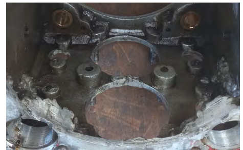
The original crankcase was distorted, cracked, and badly repaired.
