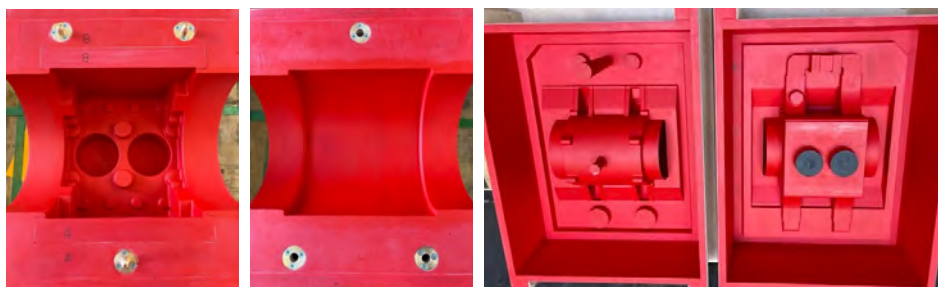
New sand casting patterns were created for the crankcase
