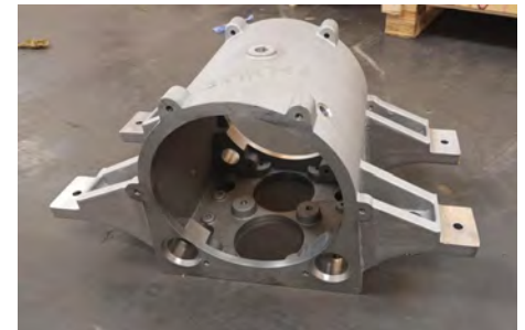
The new crankcase was cast in aluminium, heat treated and machined to the original specifications.
