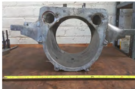
The original crankcase was distorted, cracked, and badly repaired.
